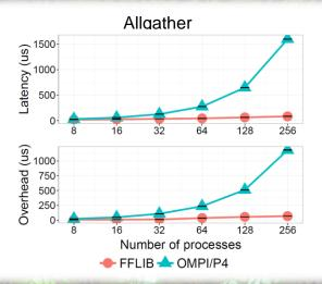
**Target machine: Curie** 5,040 nodes 2 eight-core Intel Sandy Bridge processors Full fat-tree Infiniband QDR OMPI/P4: Open MPI 1.8.4 + Portals 4 RL FFLIB: proof of concept library
