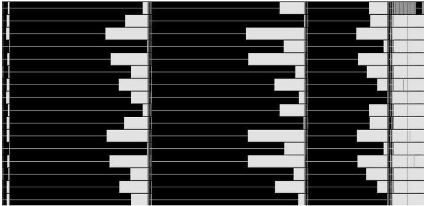
**Fig. 5.** Visualization of the MPI overhead for  $k$ -point parallelization over 16  $k$ -points on 16 Processors. Each MPI operation corresponds to a different shade of gray: `MPI_Barrier` white, `MPI_Bcast` light gray, and `MPI_Allreduce` dark gray. The synchronization overhead is much bigger than in Fig. 4. This is due to the occurring process skew.
