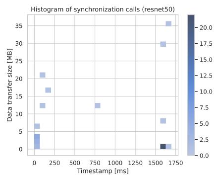
Figure 4.1: Histogram of synchronization calls in resnet50 image recognition inference (cold start)
