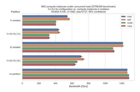
Figure 6.1: Performance isolation for compute instances in MIG under STREAM benchmark
