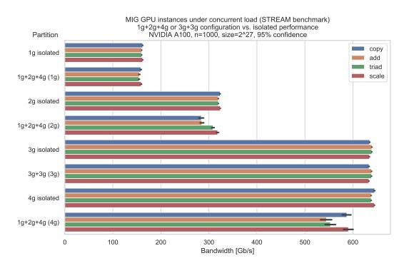
Figure 6.2: Performance isolation for GPU instances in MIG under STREAM benchmark
