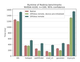
Figure 6.3: GPUless execution time vs. native in Rodinia benchmark
