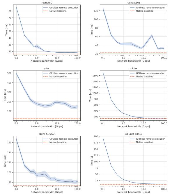
Hot model inference latency under bandwidth limitation NVIDIA RTX 3060, Intel i7-9700KF, n=100, 95% confidence
