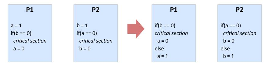
Hardware can reorder, assume a writes go to write buffer or speculation
