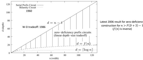
From Zhu et al.: "Construction of Zero-Deficiency Parallel Prefix Circuits", 2006
