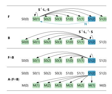
**Figure 5.** The relations of the forward map **F** and the backward map **B** for the statement instance S1(2) of the example program (the forward map **F** corresponds to the concatenation of the blue backward arrow and the black forward arrows). The map intersection defines the statement instance between and including the two accesses of M(1). The concatenation with the map **A** yields the related memory accesses.
