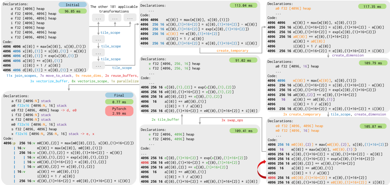
Figure 4: Optimization of a softmax kernel through a sequence of transformations (moves) on a CPU with AVX-512 extensions. Each move in the PerfDojo game maintains the initial program semantics.
