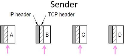
Four segments, each with 512 bytes of data and carried in an IP packet
