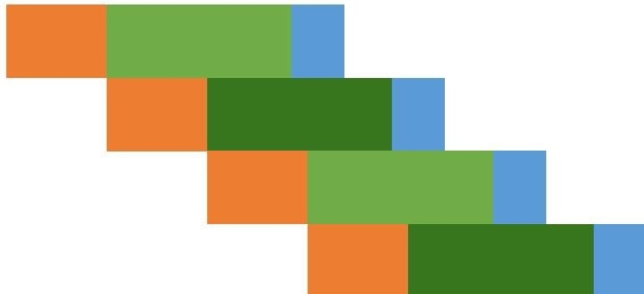
Pipeline is balanced even though the stages do not take the same time.
