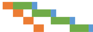
Figure 2: Pipeline executed in parallel.
