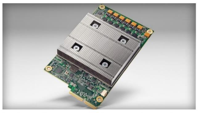
Several years ago, Google began working on its own custom software for machine learning and artificial intelligence workloads, dubbed TensorFlow. Last year, the company announced that it had designed its own tensor processing unit (TPU), an ASIC designed for high throughput of low-precision arithmetic. Now, Google has released some performance data for their TPU and how it compares to Intel's Haswell CPUs and Nvidia's
