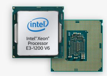
The high-end E3 v6 parts will have a maximum base frequency of 3.9 GHz base and a 4.2 GHz turbo. All the parts listed have a full 8MB of L3 cache, and either be 72W for non-IGP models or 73W for IGP parts. As with other previous Xeons, these come with ECC memory support, vPro and other technologies Intel files under the professional level. In Intel® presentations, Intel SGX (Software Guard Extensions) are included, however TSX (Transactional Extensions) were not listed.
