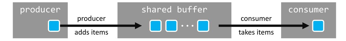
For simplicity, buffer is unbounded (has no capacity limit); producing is always possible
